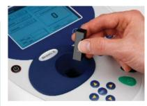
particularly useful, especially for RNA samples where impurities may be present in the 230 nm region, yet not have an adverse effect on the A260/A280 ratio. The system is compatible with disposable low volume UV cuyettes
