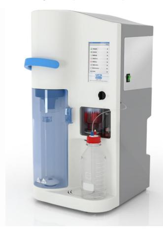
The UDK 159 Distillation & Titration System is designed to perform nitrogen and protein content according to the Kjeldahl Method (TKN) in the Food & Feed industries and several other applications in environmental control (phenols, nitrogen in water, sludge, soil and lubricant) and also in the chemical and pharmaceutical industries after having digested the sample accurately.
